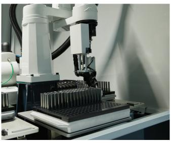
The CPX machine is offered with ANCA's own AR300 low cost loader for automated loading of tool blanks.
